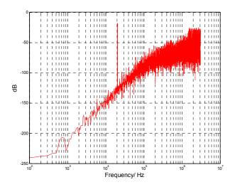
Figure 5: DAC output spectrum with the 3<sup>rd</sup> order setting.
