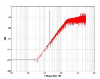
Figure 19:  $5^{th}$  order, 24-bit, SNR=139.2924dB, input=0.525, fin=20kHz, fs=96Khz, oversampling ratio=64x
