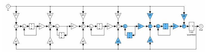
Figure 4. Architecture of the re-configurable 5<sup>th</sup>/3<sup>rd</sup> order sigma-delta modulator.
