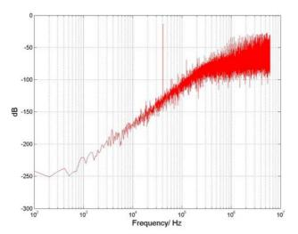
Figure 17:  $3^{rd}$  order, 24-bit SNR=98.2088dB, input=0.85, fin=20kHz, fs=96Khz, oversampling ratio=64x
