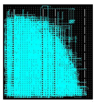
Figure 15. Place & Route Floorplan of the completed 5<sup>rd</sup> order design on Xilinx Virtex II XC2V1000, RC200
