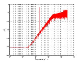
Figure 6: DAC output spectrum with the 5<sup>th</sup> order setting.
