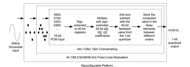
Figure 9. Sigma Delta Modulator Implementation.
