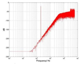
Figure 20:  $5^{th}$  order, 24-bit, SNR=171.8071dB, input=0.525, fin=20kHz, fs=96Khz, oversampling ratio=128x
