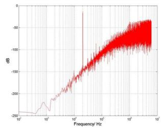
Figure 18: 3<sup>rd</sup> order, 24-bit, SNR=115.9667dB, input=0.85, fin=20kHz, fs=96Khz, oversampling ratio=128x
