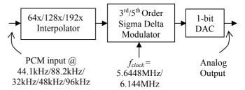
Figure 1: Block diagram of the audio DAC.
