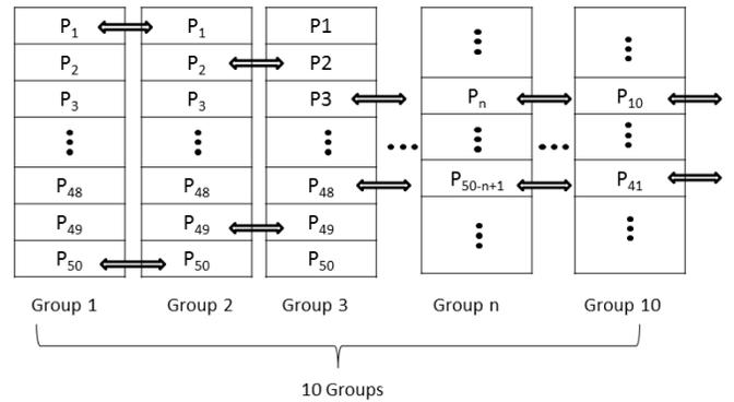
Figure 3. Illustration of deterministic mixing. There are ten groups of 50 particles each and two particles from a group are swapped with two particles in the adjacent group. First and last groups are assumed adjacent.
