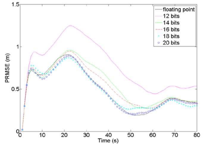
Figure 8. Effect of precision on location error ( $M=10$ ).
