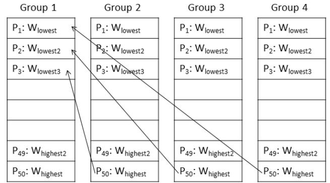
Figure 2. Illustration of lowest weight replacement mixing. There are four groups of 50 particles each and the highest weighted particles from groups two to four replaces the lowest weighted three particles from group 1.
