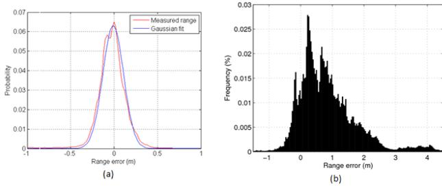
Figure 1. Range measurement noise characteristics in (a) outdoor and (b) indoor environments. Outdoor error can be approximated well with a Gaussian distribution, whereas the indoor distribution is symmetric and biased.
