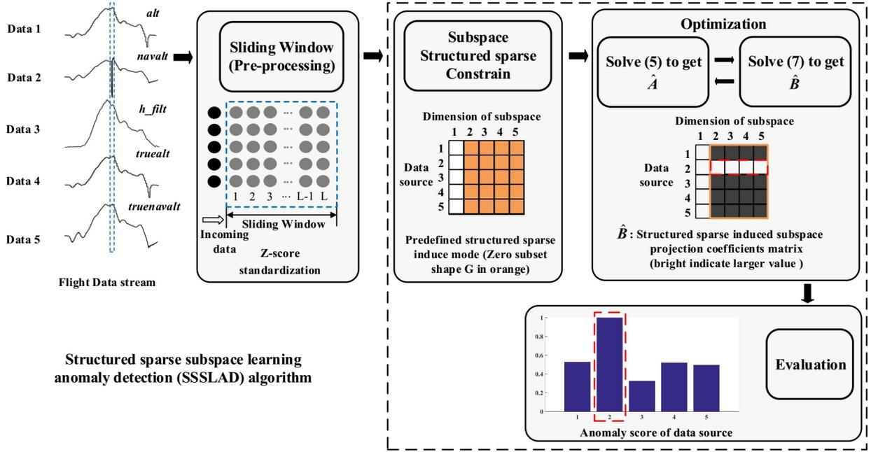
Fig. 2. Framework of structured sparse subspace learning anomaly detection (SSSLAD) algorithm.
