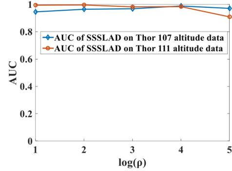
Fig. 9. AUC comparison of SSSLAD at different sparsity regularizing parameter  $\rho$  on Thor 107 and Thor 111 altitude data.
