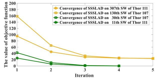
Fig. 11. Convergence of SSSLAD for different sliding windows of Thor 107 and Thor 111 altitude data.
