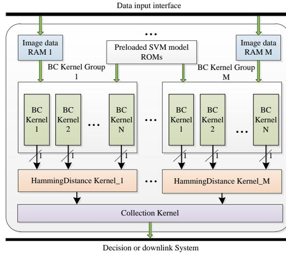
**Fig. 2.** Architecture of multi class classifier for HSI classification
