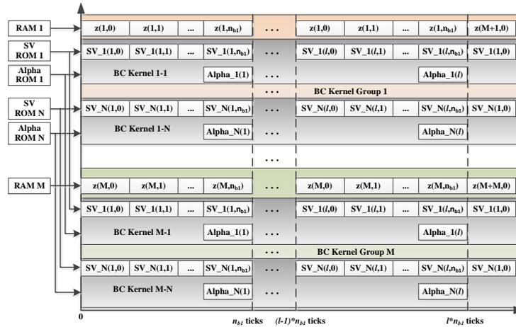
**Fig. 3.** Data flow in DFE with  $M$  classifiers and  $N$  BC kernel in each classifier
