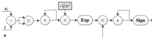
**Fig. 4.** Data path of binary classifier kernel
