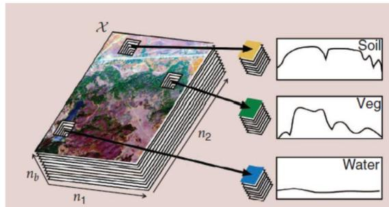
**Fig. 1.** Hyperspectral image data cube[1]
