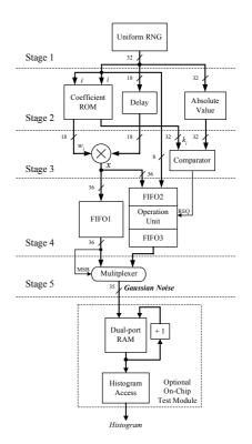
**Fig. 1.** Block diagram showing the architecture of the GRNG with optional on-chip test module. Horizontal dashed lines indicate pipeline registers and the bit-width of each bus is also shown.
